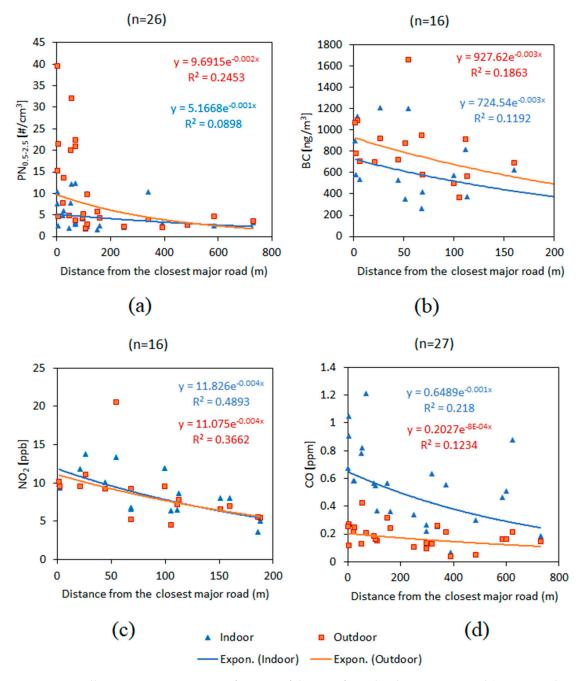
**Figure 8.** Pollutant concentrations as a function of distance from the closest major road (exponential curve-fitting) for (a)  $PN_{0.5-2.5}$ , (b) BC, (c)  $NO_2$ , (d) CO. This dataset does not include the three homes with gas stoves.
