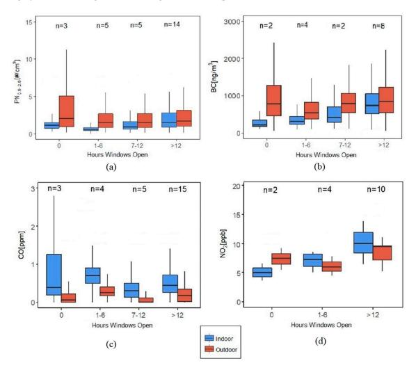
**Figure 11.** Indoor and outdoor pollutant concentration distributions (not showing outliers) according to the hours of window opening (filtered dataset) for (a)  $PN_{0.5-2.5}$ , (b) BC, (c) CO and (d)  $NO_2$ . The indoor and outdoor mean concentrations were significantly different across all window opening intervals for all pollutants except for  $NO_2$  (K-W test at  $\alpha = 0.05$ ).
