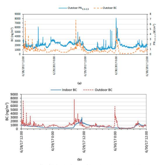
**Figure 6.** Time series profiles of black carbon from one of the test homes (Home ID: T109). (a) Compares the outdoor concentration profiles of black carbon (BC) and  $PN_{0.5-2.5}$ , and (b) compares the indoor and outdoor BC profiles.
