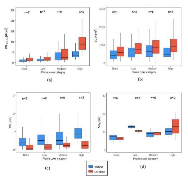
**Figure 10.** Indoor and outdoor pollutant concentration distributions (not showing outliers) according to wildfire plume cover (filtered datasets) for (a)  $PN_{0.5-2.5}$ , (b) BC, (c) CO and (d)  $NO_2$ . The indoor and outdoor concentrations between all plume categories were significantly different for all pollutants except  $NO_2$  (K-W test at  $\alpha = 0.05$ ).
