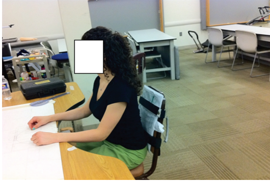
FIGURE 1: TRT workstation with sensor pad placed on anterior surface of chair back.
