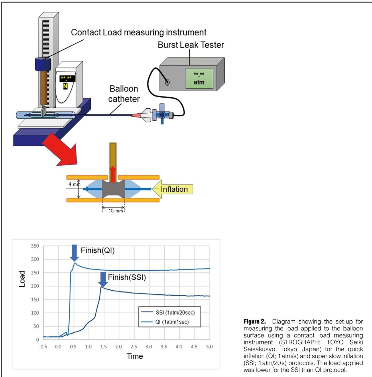
**Figure 2.** Diagram showing the set-up for measuring the load applied to the balloon surface using a contact load measuring instrument (STROGRAPH; TOYO Seiki Seisakusyo, Tokyo, Japan) for the quick inflation (QI; 1 atm/s) and super slow inflation (SSI; 1 atm/20 s) protocols. The load applied was lower for the SSI than QI protocol.
