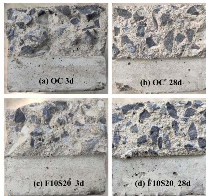
Figure 8. Fracture surfaces of OC and F10S20 concrete specimens: (a) OC concrete at 3 d; (b) OC concrete at 28 d; (c) F10S20 concrete at 3 d; (d) F10S20 concrete at 28 d.
