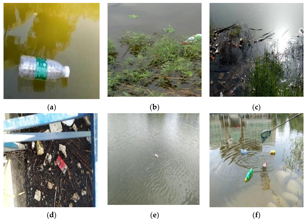
Figure 5. Float debris images with various disturbance: (a) ideal detection target; (b) blocked target; (c) strong reflection; (d) complex water surface; (e) small target; (f) ripples.
