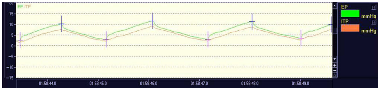
Fig. 4. Typical graph of intratracheal pressure (ITP) course as measured through the stylet placed 2 cm above the carina during ventilation with Ventrain in a sealed airway run (screen shot from the data acquisition system). Note the linear inspiratory pressure increase as well as the linear expiratory pressure decrease.
