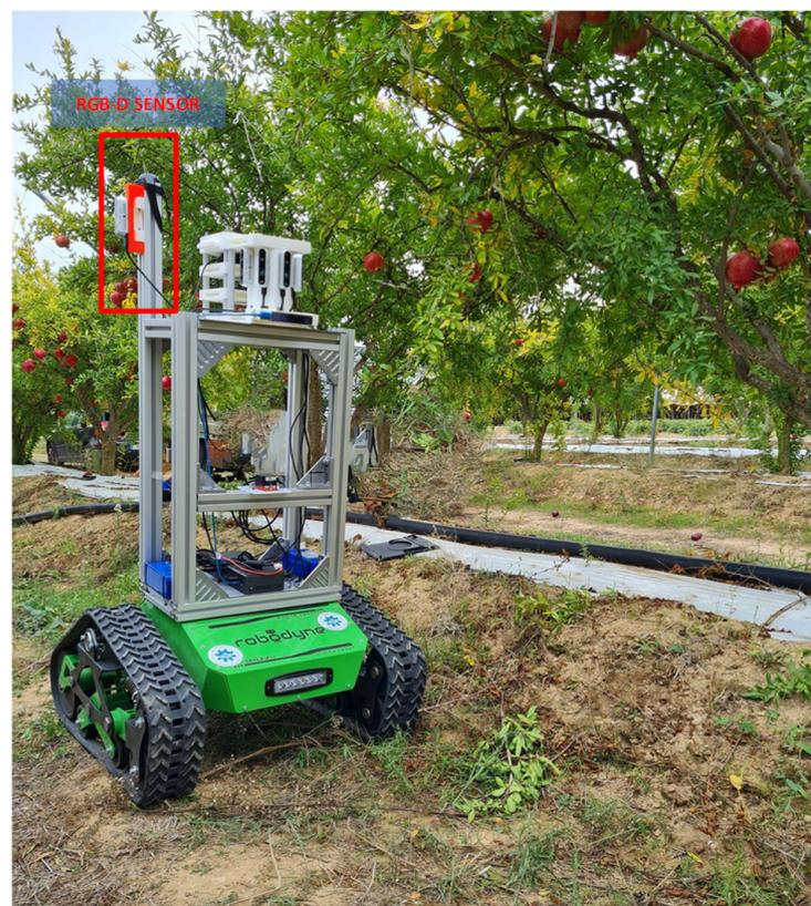
**Figure 1.** The farmer robot, Polibot, used for experimentation, equipped with a multi-sensor suite.
