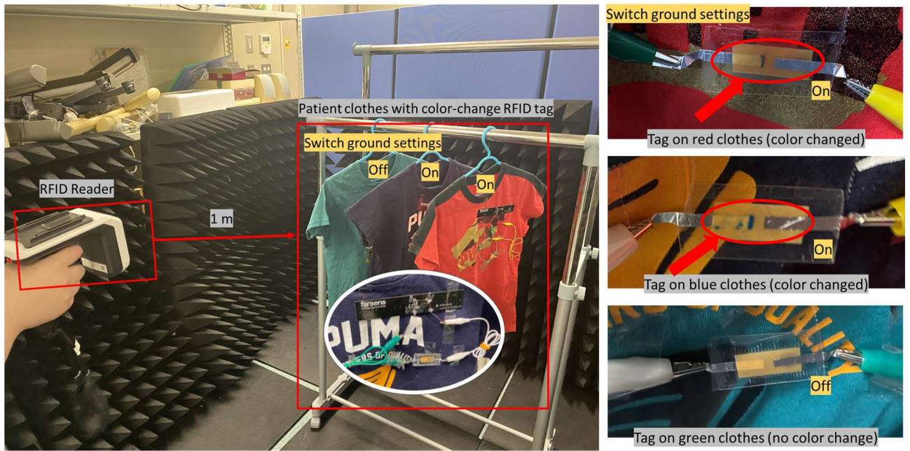
Figure 2. Demonstration of IoMT application for managing patient clothes after 30 s of management (RFID reader irradiation). The red and blue clothes are set as the target clothes (Switch ground setting = ‘on’). The color-change positions are specified by red arrows and circles.
