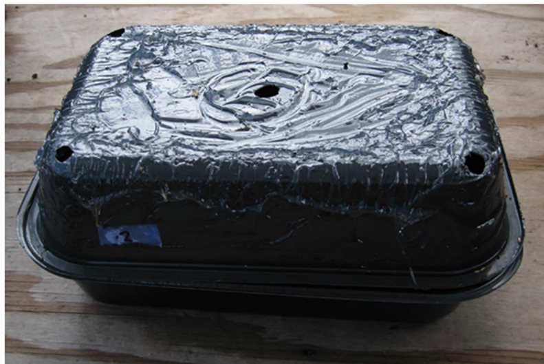
Fig 1. Presentation of concealed fruit (placed inside the two inverted black plastic containers) that was sliced to release induced volatiles. The top container was coated with Tangletrap to capture alighting female B. cucurbitae . Four holes in the corners of the top container and one at the center allowed diffusion of host fruit volatiles.
