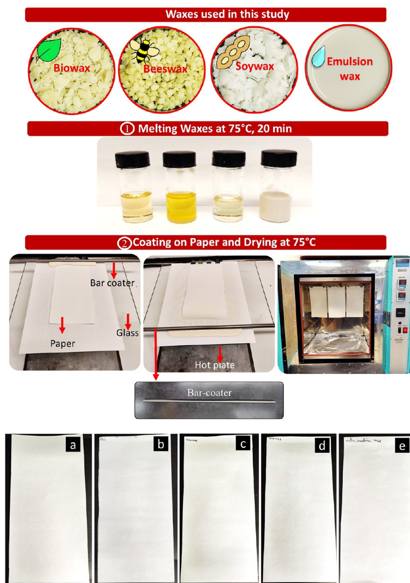
Figure 1. Experimental methodology; preparation of waxes and coating on the paper. The natural appearance of waxes as well as the molten waxes and wax-coated papers is shown: (a) uncoated paper and (b) biowax-, (c) beeswax-, (d) soywax-, and (e) emulsion wax-coated paper. The emulsion wax is shown as an example for the coating process.
