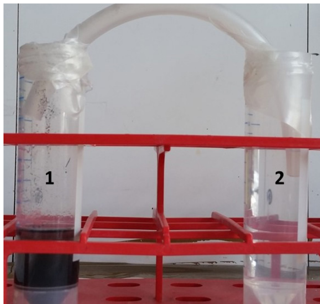
FIGURE 3. Set-up for testing microbial catalase activity in soil (Exercise 3). Tube 1: soil mixed with hydrogen peroxide solution. Tube 2: 30–40 mL water.
