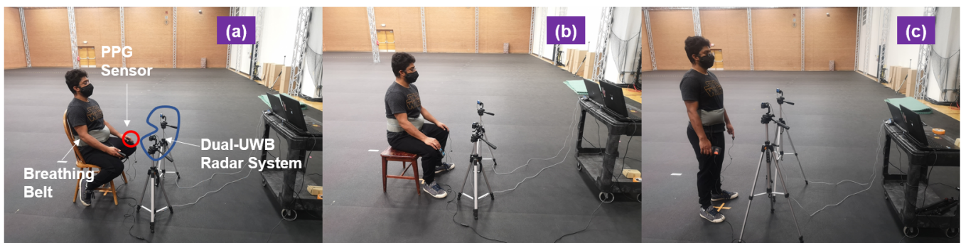
Figure 1. Novel dual-UWB radar system same-side scenario. (a) Stable seating; (b) free-style seating; (c) standing.
