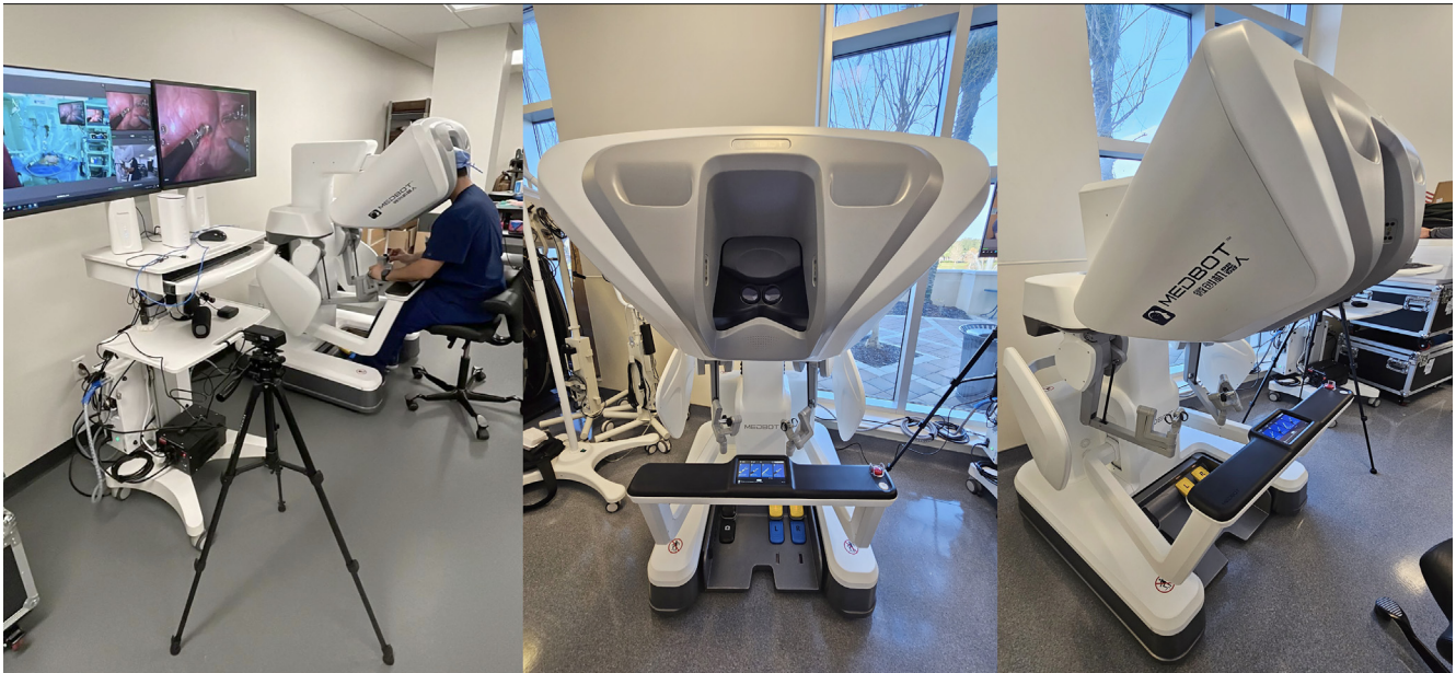
Fig. 1 – Toumai robotic console in Orlando and the connection setup with the animal laboratory in Shanghai.
