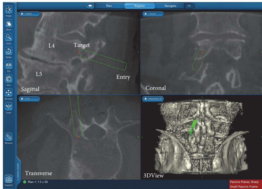
FIGURE 4: Screenshot taken from the StealthStation navigation system. The display that a surgeon has access to during a procedure is shown. The location of each vertebra, the screw trajectory coordinates, and the anatomical planes are marked in this figure, but are not during the procedure. This image was obtained from the workstation's spinal software.
