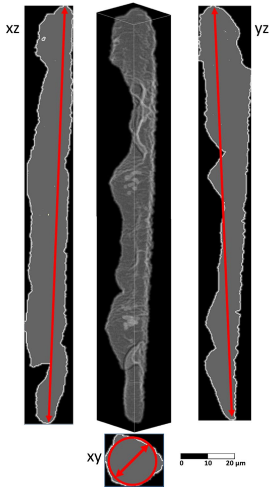
Figure 8. The 3D reconstruction of a sub-element void of S19 sample. The projections of the void are shown in grey. The length of the voids is estimated using the major axes of the projections on XZ and YZ planes, while the void diameter was calculated from the circle equivalent to the projection on the plane XY. The image was generated by using the Fiji distribution of ImageJ 40 . [ImageJ-1.53c https://imagej.net/ImageJ ].
