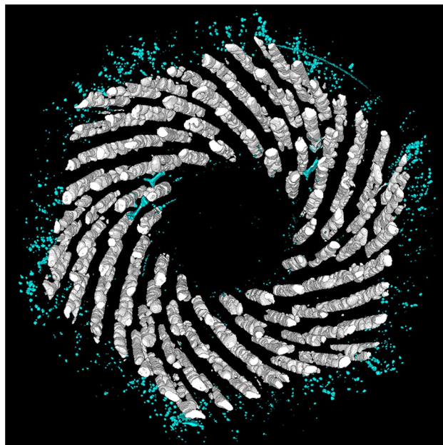
Figure 3. The 3D voids reconstruction of the sample S20. The voids in the sub-elements are white while the copper voids are light blue. The image was generated by using the Fiji (Fiji is Just ImageJ) distribution of ImageJ 40 . [Image]-1.53c https://imagej.net/ImageJ ].
