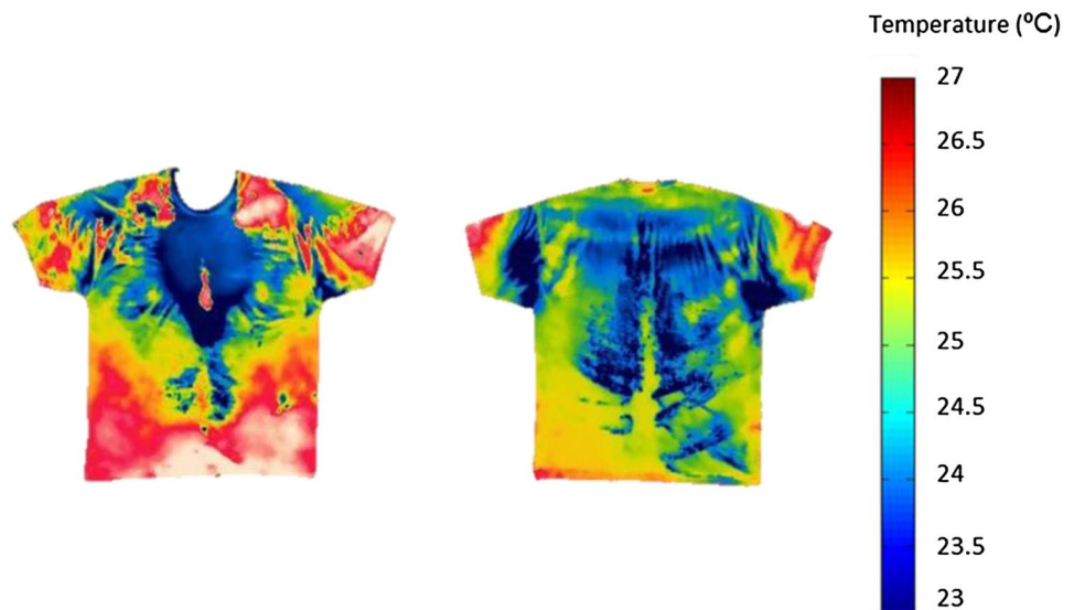
Fig. 3 Example of infrared pictures of front and back of the T-shirt after 30 min of running exercise taken to identify variations in sweat retentions between various T-shirt regions
