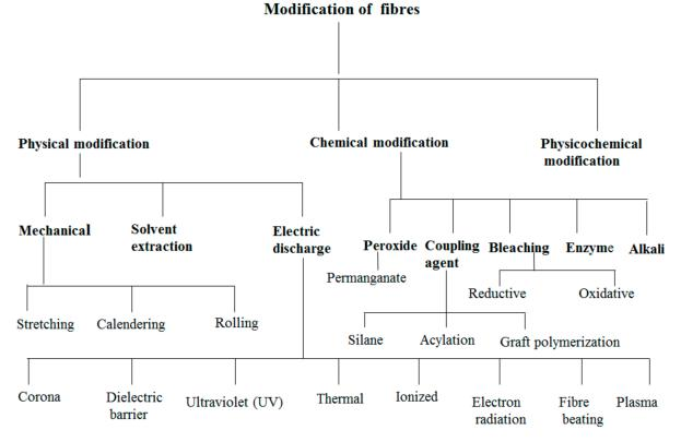
Figure 10. Different methods for fiber modification.
