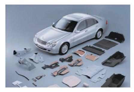
**Figure 4.** Automobile components fabricated with natural fiber related composites. Reprinted with permission from the publisher [16]. Open access.
