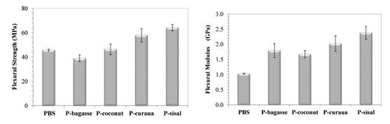
**Figure 18.** Flexural strength and modulus of PBS and its natural fiber-reinforced composites. Reprinted with permission from the publisher [131].
