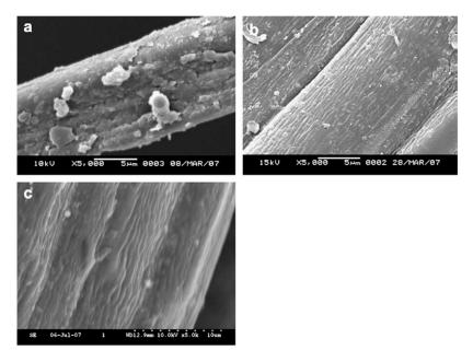
**Figure 11.** Surface modification of the fiber: (**a**) no modification, (**b**) alkali, and (**c**) coupling treatments. Reprinted with permission from Elsevier [103].
