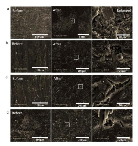
**Figure 19.** SEM images of pure PBS and sugarcane rind fiber (SRF)/PBS composites at various SRF contents before and after 100 days of soil burial: (**a**) pure PBS, (**b**) 5 wt.% SRF, (**c**) 10 wt.% SRF and (**d**) 15 wt.% SRF [143]. Copyrights obtained from Elsevier.
