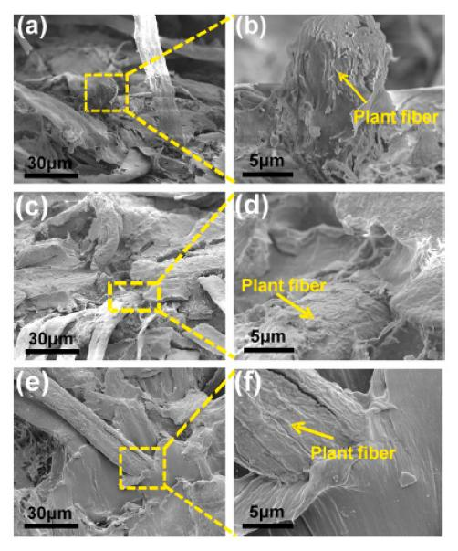
**Figure 15.** SEM of waste paper (WP)/PBS composites at various WP contents after flexural fracture: (a) and (b) 10 wt.% WP, (c) and (d) 30 wt.% WP, and (e) and (f) 60 wt.% WP [125]. Copyrights obtained from Elsevier.
