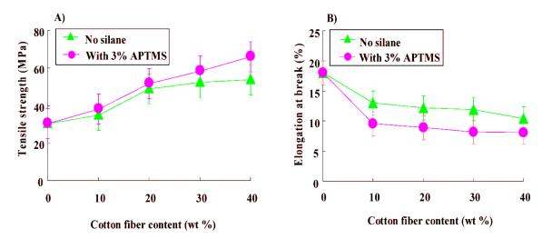
**Figure 17.** (a) Tensile strength and (b) elongation at break for PBS/cotton fiber (treated and untreated) [127]. Reprinted with permission from the publisher. Open access.
