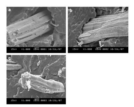
**Figure 12.** Surface morphology of (**a**) untreated jute/PBS, (**b**) alkali-treated jute fiber/PBS and (**c**) coupling-treated jute fiber/PBS biocomposites. Reprinted with permission from Elsevier [103].
