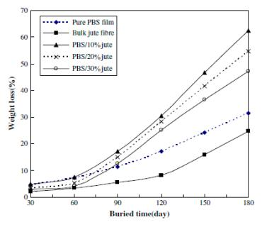
**Figure 20.** Weight loss of buried pure PBS film, bulk jute fiber and PBS/jute fiber composites at various fiber contents [103]. Elsevier.
