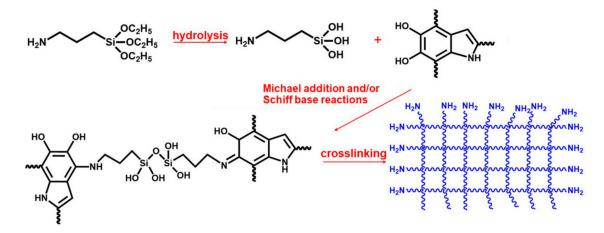
**Figure 14.** A scheme illustrating the modification of the fiber, a reactive mechanism between modifiers and the fabrication of the biocomposites. Reprinted with permission from Elsevier [124].
