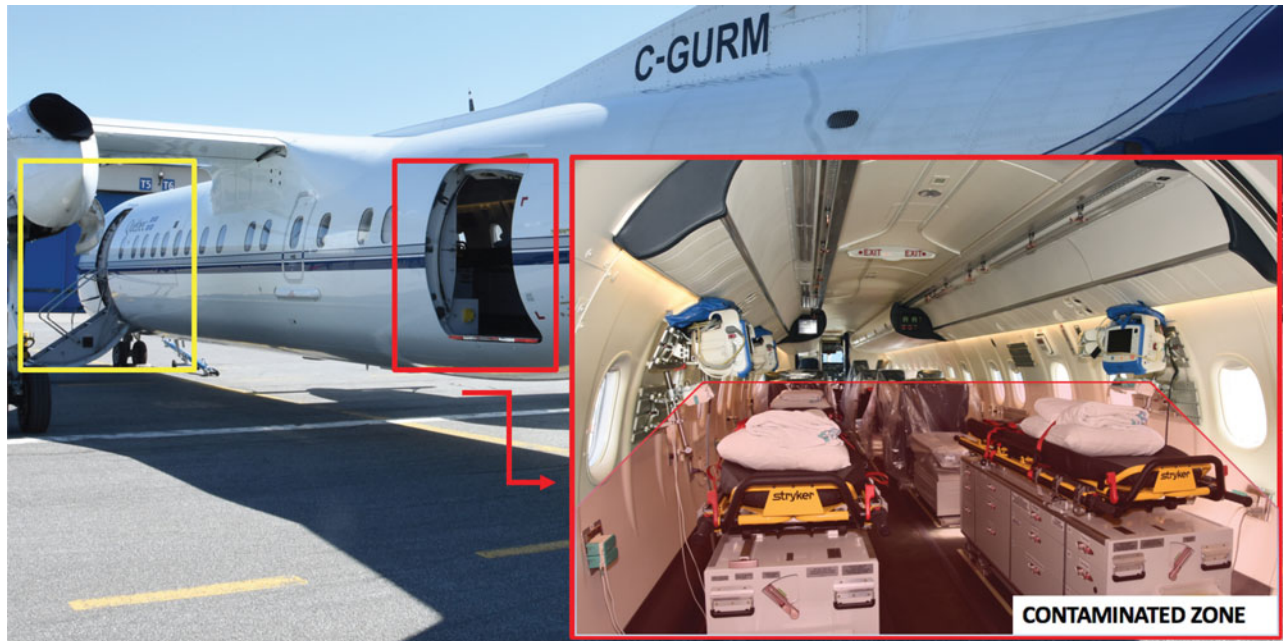
Figure 1. Representation of boarding zones for the aircraft, whereby uncontaminated personnel board through the front door (yellow), and patients and treating medical staff board through the cargo door (red). This allows for safe transition zones within the airplane (De Havilland Canada DHC-8, Service d'évacuation aéromédicales du Québec).
