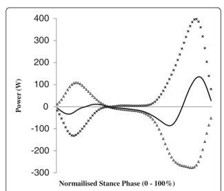
Figure 1 Exemplar trial showing stance phase net power (P<sub>dist</sub> solid line) along with the rotational prosthetic power (P<sub>rot</sub>, triangles) and translational joint power (P<sub>trans</sub>, crosses) at the distal end of the prosthetic shank (*pros end*). Negative values indicate power leaving the shank (flow to the foot) and positive values indicate power entering the shank (flow from the foot).
