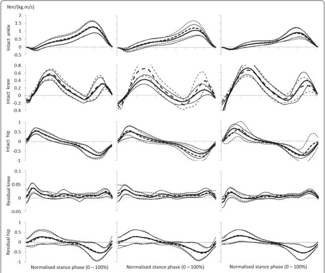
Figure 2 Ensemble mean (± 1 SD) speed normalised stance phase moments at the hip, knee and ankle (intact limb only) joints when using rigid (rigF, dotted lines) and hydraulic (hyA-F, solid lines) ankle-foot devices at slow (left column), customary (centre column) and fast (right column) speed levels.
