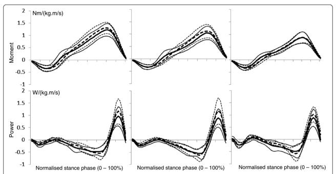
Figure 4 Ensemble mean (± 1 SD) speed normalised stance phase external moment (plantarflexion – negative, dorsiflexion – positive) and power profiles at *pros end* when using rigid (*rig*F, dotted lines) and hydraulic (*hy*A-F, solid lines) ankle-foot devices at slow (left column), customary (centre column) and fast (right column) speed levels. Negative power is power leaving the shank into the foot and positive power is power returning to the shank from the foot.
