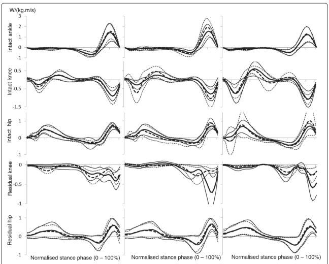
Figure 3 Ensemble mean ( $\pm$  1 SD) speed normalised stance phase muscle power generation (positive) and absorption (negative) at the hip, knee and ankle (intact limb only) joints when using rigid (rigF, dotted lines) and hydraulic (hyA-F, solid lines) ankle-foot devices at slow (left column), customary (centre column) and fast (right column) speed levels.
