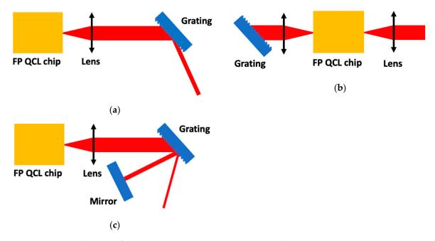
**Figure 7.** Schematic of Fabry–Pérot Quantum Cascade Laser chip source in an external-cavity system in (**a**) front facet Littrow configuration, (**b**) back facet Littrow configuration and (**c**) front facet Littman configuration.
