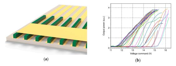
**Figure 2.** (a) Schematics of the DFB QCL array. The electrical contact (in yellow) of the DFB QCLs (in green) is given by a gold common terminal and by gold individual tracks under the lasers; (b) Power of the 34 QCLs of the array vs. voltage command. Supply conditions of all pulsed lasers are: temperature 20 °C, pulse duration 100 ns, repetition rate 100 kHz, peak current 1.3 A.
