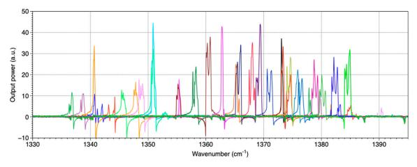
Figure 4. Emission spectra of all the QCLs from the DFB QCL array for one temperature (20 °C).
