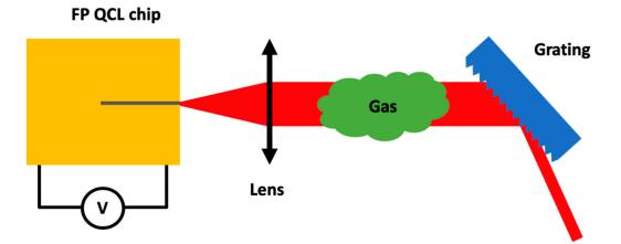
**Figure 9.** Schematic of an External Cavity Quantum Cascade Laser—Voltage Intracavity Sensing for gas detection in front facet Littrow configuration. Note that, in this case, no detection system is needed as the cavity is the light source and the detector at the same time.
