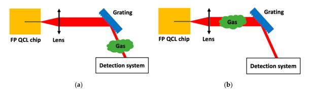
**Figure 8.** (a) Schematic of a standard Fabry–Pérot Quantum Cascade Laser chip source in an external-cavity system for gas detection in front facet Littrow configuration and (b) the same set-up used to perform Intra-Cavity Laser Absorption Spectroscopy.
