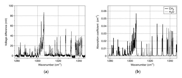
**Figure 11.** (a) Experimental spectra and (b) absorption coefficient calculated from HITRAN data assuming 0.3% of methane and 3% of water vapor in ambient air at atmospheric pressure.
