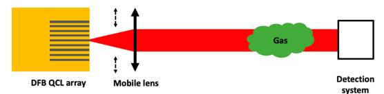
**Figure 1.** Schematic of a DFB QCL array source for gas detection. Grey lines in the yellow square indicate the lasers in the array. A mobile lens following the dashed arrows must be moved to adapt to the output of the chosen laser.
