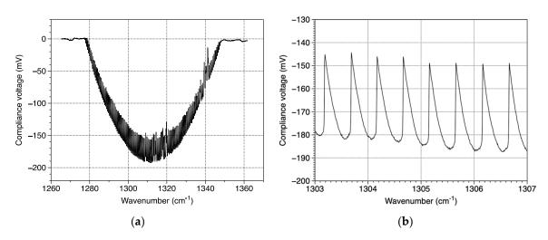
**Figure 10.** (a) QCL device compliance voltage when varying the mirror angle  $\pm 3^{\circ}$  and (b) a zoom on Figure 10a around 1305 cm<sup>-1</sup>.
