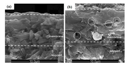
**Figure 3.** Cross-section of zeolite T membrane heated at 4.8 kW/m<sup>3</sup> (**a**) and 6.0 kW/m<sup>3</sup> (**b**); the circle indicates the area defects [11] (Reproduced with permission from Zhou et al., Microwave-assisted hydrothermal synthesis of a&b-oriented zeolite T membranes and their pervaporation properties; published by Elsevier, 2009).
