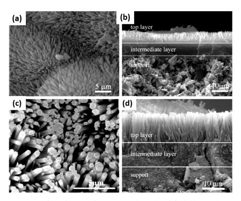
**Figure 7.** SEM for zeolite T membrane at 373 K (100 °C), 35 h for (**a**,**b**); 423 K (150 °C) for 20 h for (**c**,**d**) [5] (Reproduced with permission from Zhou et al., Synthesis of oriented zeolite T membranes from clear solutions and their pervaporation properties; published by Elsevier, 2013).
