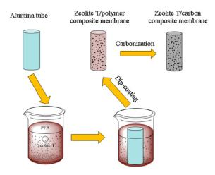
**Figure 5.** Schematic diagram of dip-coating method in preparing zeolite T/carbon composite [16] (Reproduced with permission from Yin et al., Thin zeolite T/carbon composite membranes supported on the porous alumina tubes for CO<sub>2</sub> separation; published by Elsevier, 2013).
