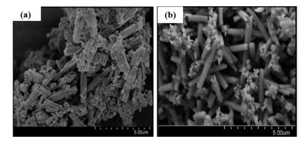
**Figure 4.** Morphology of zeolite T synthesized in 168 h without sonication (**a**), and zeolite T form in 24 h assisted with sonication pre-treatment (**b**) [12] (Reproduced with permission from Jusoh et al. Rapid-synthesis of Zeolite T via sonochemical-assisted hydrothermal growth method; published by Elsevier, 2017).
