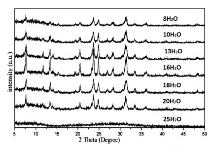
**Figure 9.** XRD spectrum or zeolite T's samples synthesized at different moles of water [3] (Reproduced with permission from Yin et al., Hydrothermal synthesis of hierarchical zeolite T aggregates using tetramethylammonium hydroxide as single template; published by Elsevier, 2015).
