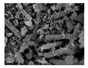
**Figure 1.** Rod-like shape of zeolite T synthesized by [3] (Reproduced with permission from Yin et al., Hydrothermal synthesis of hierarchical zeolite T aggregates using tetramethylammonium hydroxide as single template; published by Elsevier, 2015).
