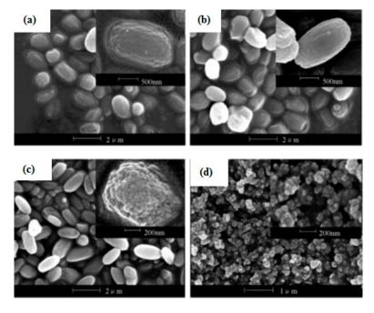
**Figure 11.** SEM images of zeolite T at 373 K (100 °C) at different amounts of TMAOH: (**a**) 0.05, (**b**) 0.10, (**c**) 0.15 and (**d**) 0.22 [3] (Reproduced with permission from Yin et al., Hydrothermal synthesis of hierarchical zeolite T aggregates using tetramethylammonium hydroxide as single template; published by Elsevier, 2015).
