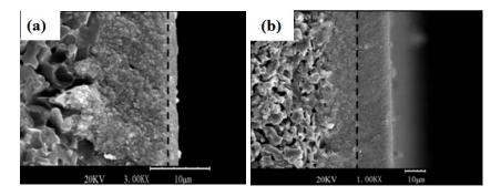
**Figure 6.** Morphology of zeolite T membrane undergone one coating cycle (**a**) and four coating cycle (**b**) [16] (Reproduced with permission from Yin et al., Thin zeolite T/carbon composite membranes supported on the porous alumina tubes for CO<sub>2</sub> separation; published by Elsevier, 2013).
