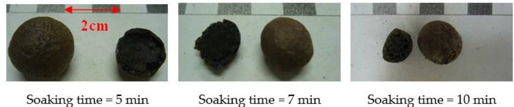
Figure 9. Appearances and profiles of the sintered LWAs during the second stage (the W30 formula).
