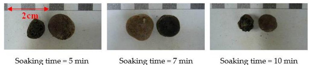
Figure 10. Appearances and profiles of the sintered LWAs during the second stage (the W50 formula).
