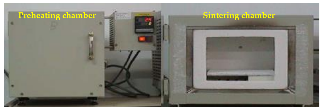
Figure 4. Programmable high-temperature electric furnace.
