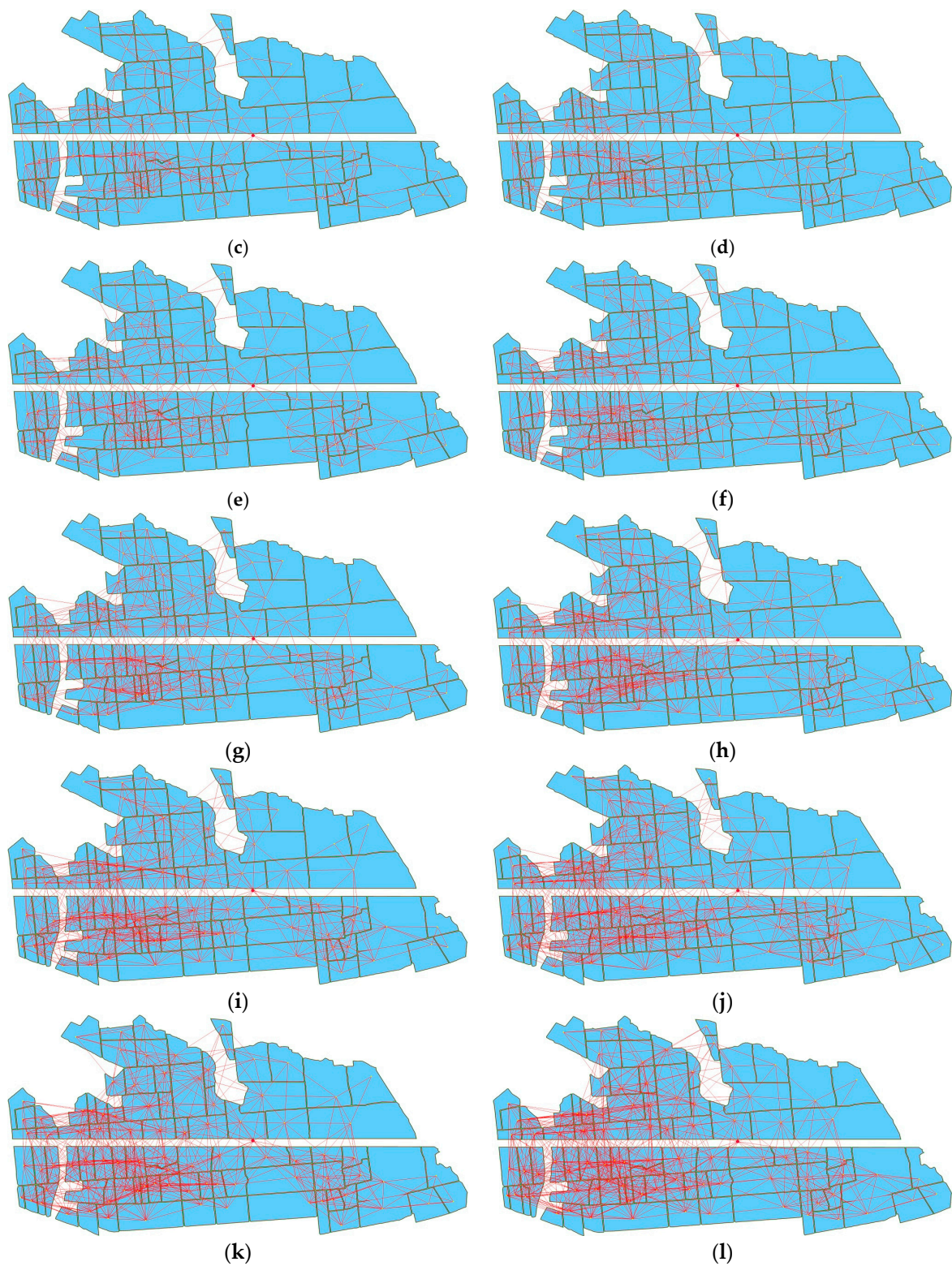
Figure 18. The WSNs deployed using method of this paper for different values of d . (a) d = 140 m; (b) d = 150 m; (c) d = 160 m; (d) d = 170 m; (e) d = 180 m; (f) d = 190 m; (g) d = 200 m; (h) d = 210 m; (i) d = 220 m; (j) d = 230 m; (k) d = 240 m; (l) d = 250 m.
