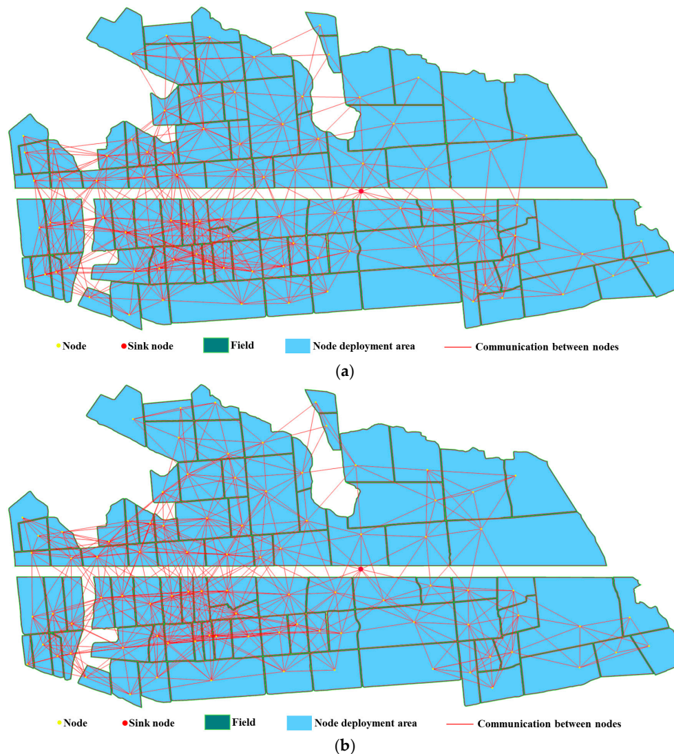
Figure 16. The WSN deployment on natural farmland located in Nanjing, Jiangsu Province, China. The communication distance is 200 m. (a) k = 3 ; (b) k = 4 .
