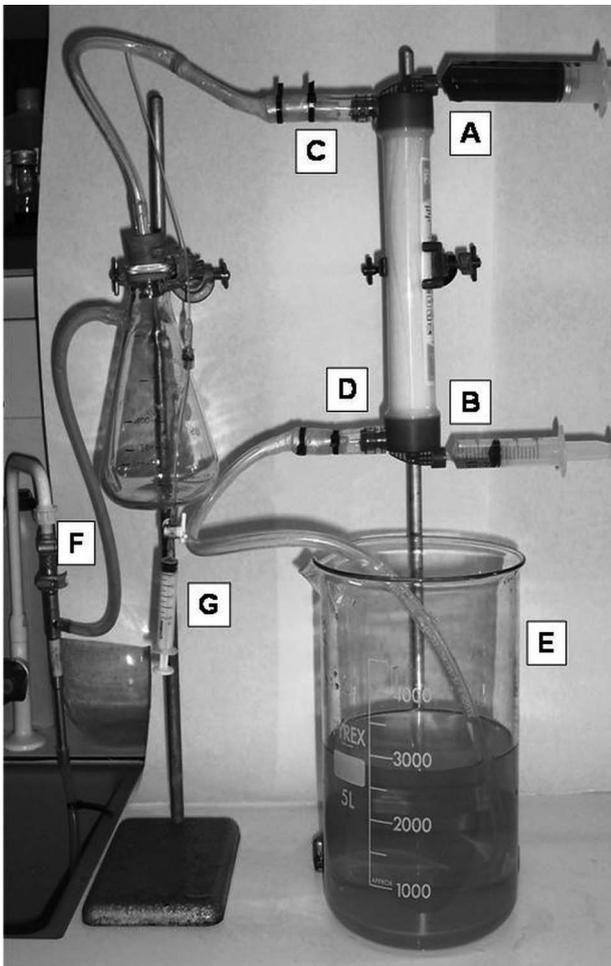
**Figure 1** In vitro setup of simulated haemodialysis. (A) Blood compartment inlet; (B) blood compartment outlet; (C) dialysate outlet; (D) dialysate inlet; (E) dialysate reservoir; (F) water-driven vacuum pump; (G) efferent dialysate collection syringe.
