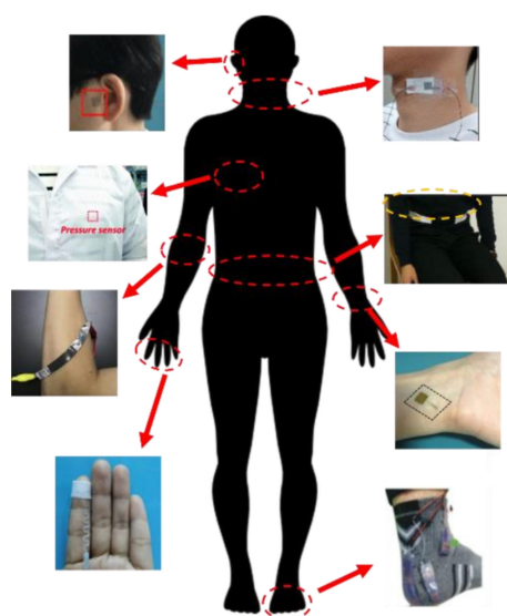
Figure 1. The detection positions for wearable pressure monitoring, such as ears [6], neck [10], arms [13], waist [14], wrists [15,19], fingers [16], chest [17], and feet [18].
