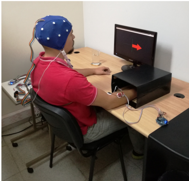
Fig. 5. Experiment set-up. The subject seated in front of a computer screen, where the stimulation protocol was being presented. The EEG cap was connected to the OpenBCI Cyton + Daisy board and the EMG Myoware electrodes were connected to the OpenBCI Ganglion board. Each board was wirelessly connected to a dedicated PC.
