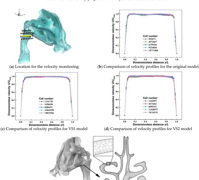
(e) Final unstructured polyhedral mesh with prism layers for the original model
