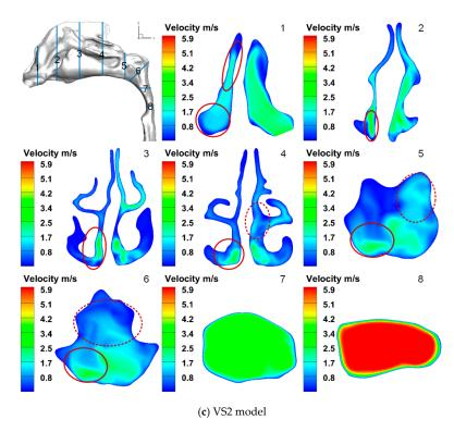
Figure 3. Velocity distributions of cross-sections of the nose-to-throat models at 15 L/min.
