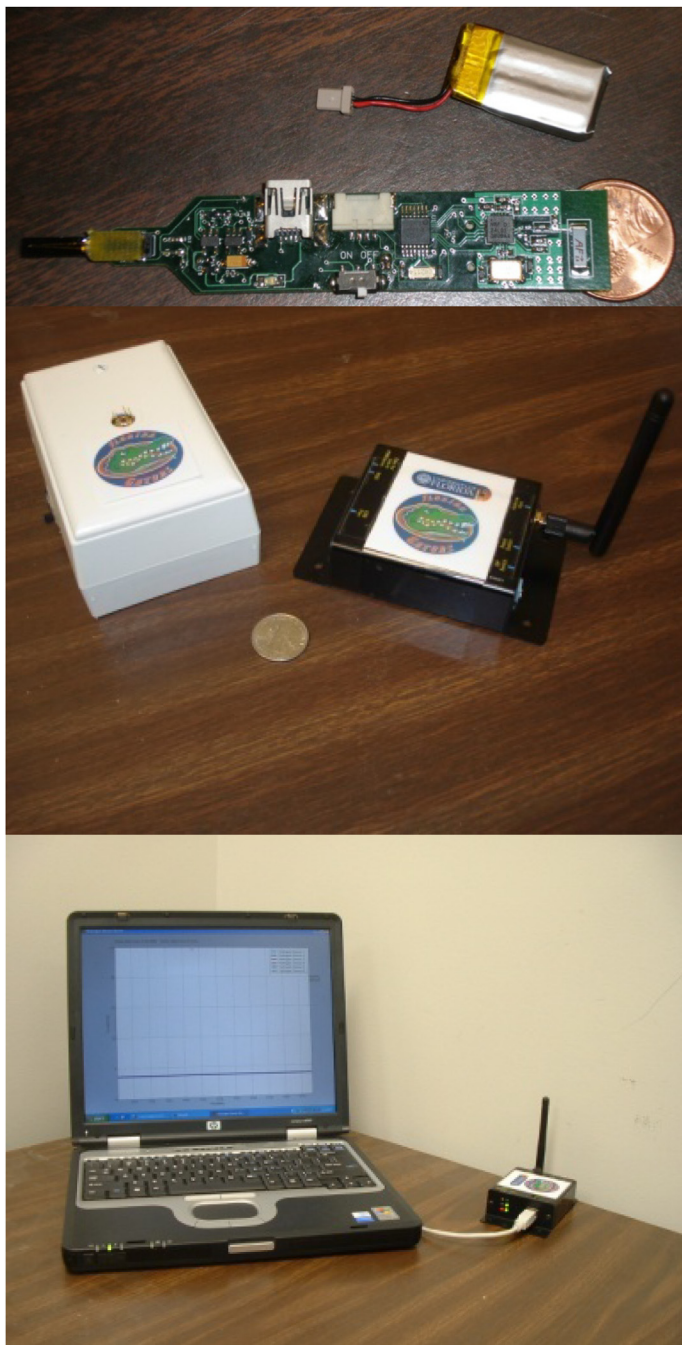
FIGURE 24.10 Photographs of integrated pH sensor (top) and receiver/transmitter pair (center) and connection to computer (bottom).
