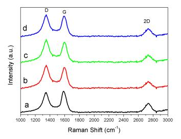
**Figure 4.** Raman spectra of thermally treated Fe-lignin samples prepared using different iron sources as catalysts: Fe-N (a), Fe-Cl<sub>3</sub> (b), Fe-Cl<sub>2</sub> (c) and Fe-S (d).
