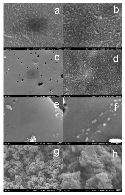
**Figure 5.** Scanning electron microscope images of four iron source (iron(II) sulfate (a,b) iron(II) chloride (c,d), iron(III) chloride (e,f) and iron nitrate (g,h)) promoted kraft lignin samples thermally treated at 1000 °C for 1 h under an argon flow.
