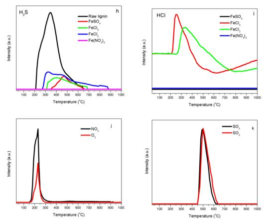
**Figure 2.** Evolution of gases and volatiles from thermally treated kraft lignin samples promoted with different iron compounds (FeCl<sub>2</sub>, FeCl<sub>3</sub>, FeSO<sub>4</sub> and Fe (NO<sub>3</sub>)<sub>3</sub>): (a)  $H_2$ , (b)  $CH_4$ , (c) CO, (d)  $CO_2$ , (e) phenol, (f) benzene, (g)  $CH_3OH$ , (h)  $H_2S$ , (i) HCl (from FeCl<sub>2</sub>, FeCl<sub>3</sub>), (j)  $NO_2$  and  $O_2$  (from Fe (NO<sub>3</sub>)<sub>3</sub>), (k)  $SO_2$  and  $SO_3$  (from FeSO<sub>4</sub>).
