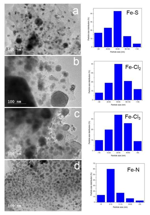
**Figure 6.** High resolution transmission electron microscope images of four iron sources (iron(II) sulfate (a) iron(II) chloride (b), iron(III) chloride (c) and iron nitrate (d)) promoted kraft lignin after thermal-treated at  $1000\,^{\circ}\text{C}$  for 1 h under an argon flow.
