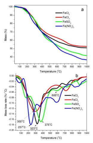
**Figure 1.** TG (**a**) and DTG (**b**) curves of kraft lignin promoted with four iron salts: FeCl<sub>2</sub>, FeCl<sub>3</sub>, FeSO<sub>4</sub> and Fe (NO<sub>3</sub>)<sub>3</sub>.
