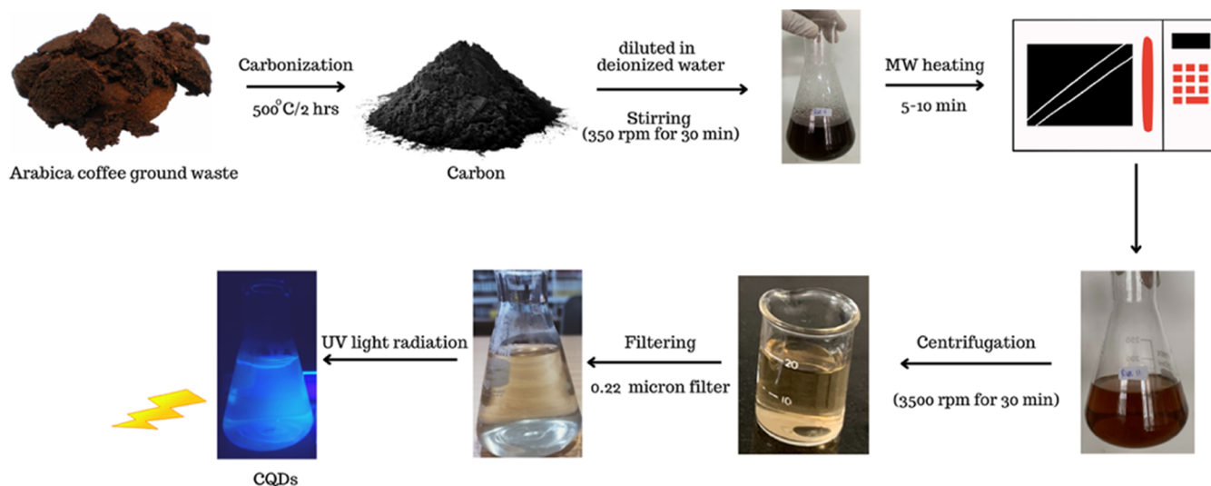
Figure 1. Schematic illustration for fabrication of CQDs via microwave heating.
