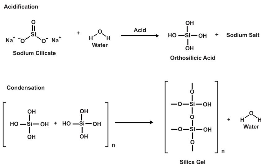
Fig. 1. Acidification and condensation of sodium silicate.
