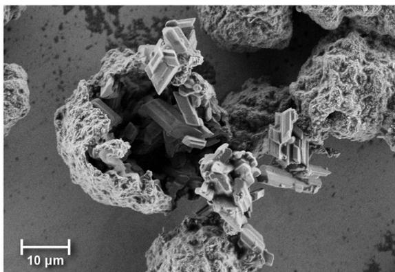
**Fig. 10.** A fractured tretinoin Microcapsule displaying the core shell structure, revealing the inner tretinoin crystals (A) within the silica shell (B).
