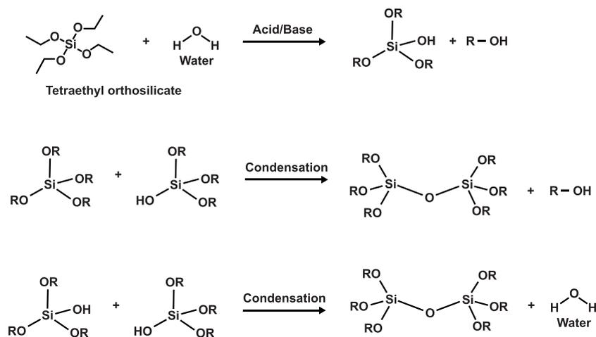
Fig. 2. Hydrolysis and condensation of alkoxides.
