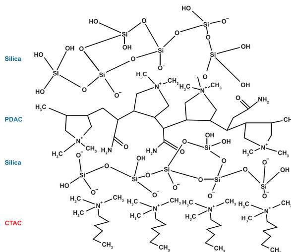
Fig. 3. A Schematic Representation of the Chemical Interactions Between CTAC, Silica, and PDAC in the Shell. CTAC, cetyltrimonium chloride; PDAC, polyquaternium-7.
