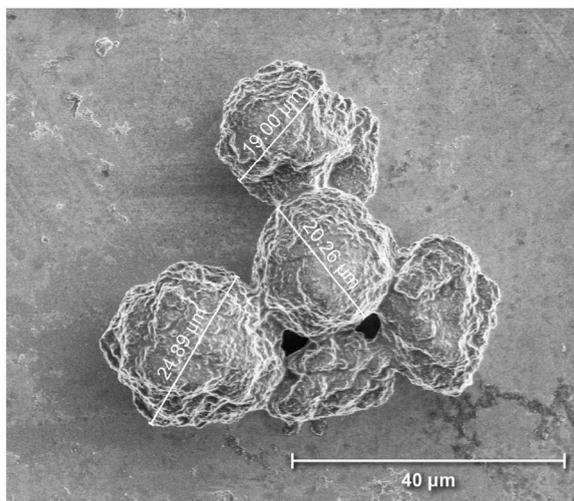
**Fig. 9.** Tretinoin Microcapsule image under scanning electron microscopy.
