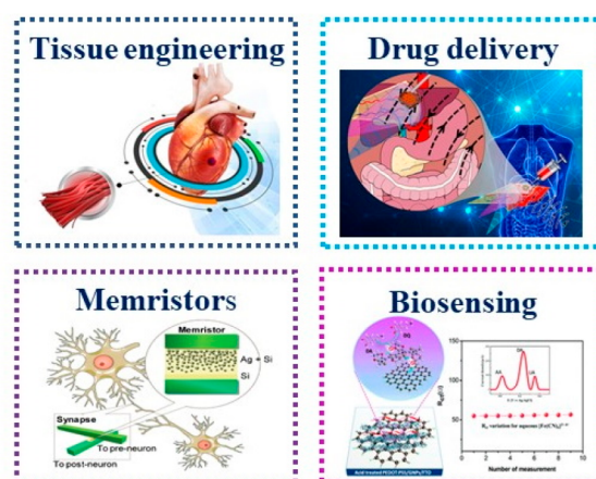
Figure 1. Applications of bioelectronics. Panel 1: Schematic of the nanomaterials utilized for the production of electrically conductive cardiac tissue engineering scaffolds. Adapted with permission from ref 22. Copyright 2019 Elsevier. Panel 2: Schematic of electromagnetically controlled drug release. Reproduced with permission from ref 23. Copyright 2019 Wiley. Panel 3: Schematic illustration of the memristors as interneuron synapses. The insets show the schematics of the two-terminal device geometry and the layered structure of the memristor. Adapted with permission from ref 24. Copyright 2010 American Society of Chemistry. Panel 4: Schematic of the removal of PSS from the PPG by \text{H}_2\text{SO}_4 treatment. Adapted with permission from ref 25. Copyright 2017 Royal Society of Chemistry.
