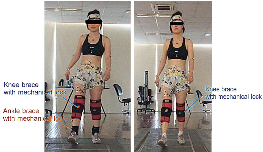
FIGURE 1: Two gaits were tested in this study. (a) Both knee and ankle immobilization (KAI) gait and (b) knee immobilization (KI) gait.
