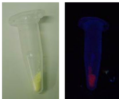
Figure S2 Ultraviolet (UV) luminescence image of silica-coated cadmium sulfide quantum dots after 3 months of normal day/night light storage to depict increased stable shelf life.
