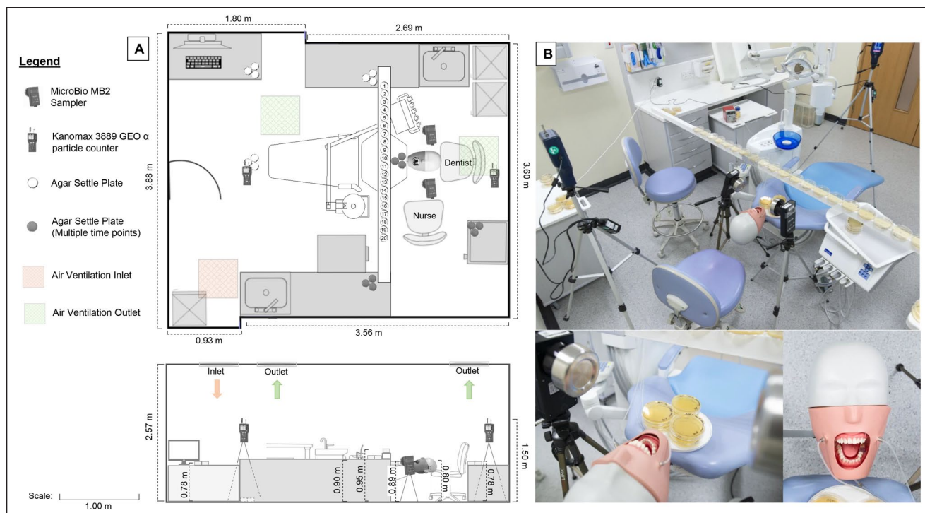
Figure 1. Experimental setup in the Leeds Dental Institute surgery. (A) Schematic of experimental setup (top, above; bottom, side view). (B) Top: photographic overview of surgical clinic layout. Bottom: closeup of the phantom head with saliva tubing inputs and oral cavity configuration.
