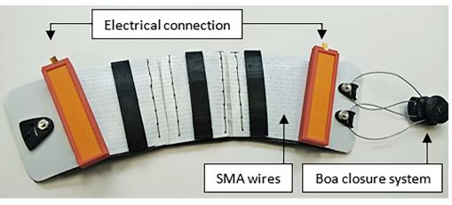
**Fig 1.** Active compression brace (ACB). The ACB consisted of thin layer of Teflon on top of a protective layer of Neoprene as the body of the brace and SMA wires as the actuators. The 3D printed guides and fixtures with the Boa closure systems, placed at the end of the brace, are also shown in the figure.
