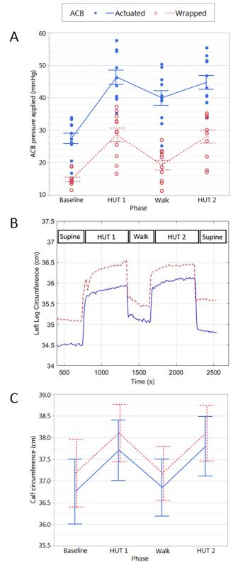
**Fig 3. ACB performance and its impact on calf circumference changes.** There was a significant main effect of ACB activation on the calf pressures obtained difference (p<0.001) (A). A representative example trace from one participant showing the impact of the ACB in wrapped and actuated conditions (B). Group data (left and right legs combined) showing the impact on calf circumference in the two experimental conditions are
