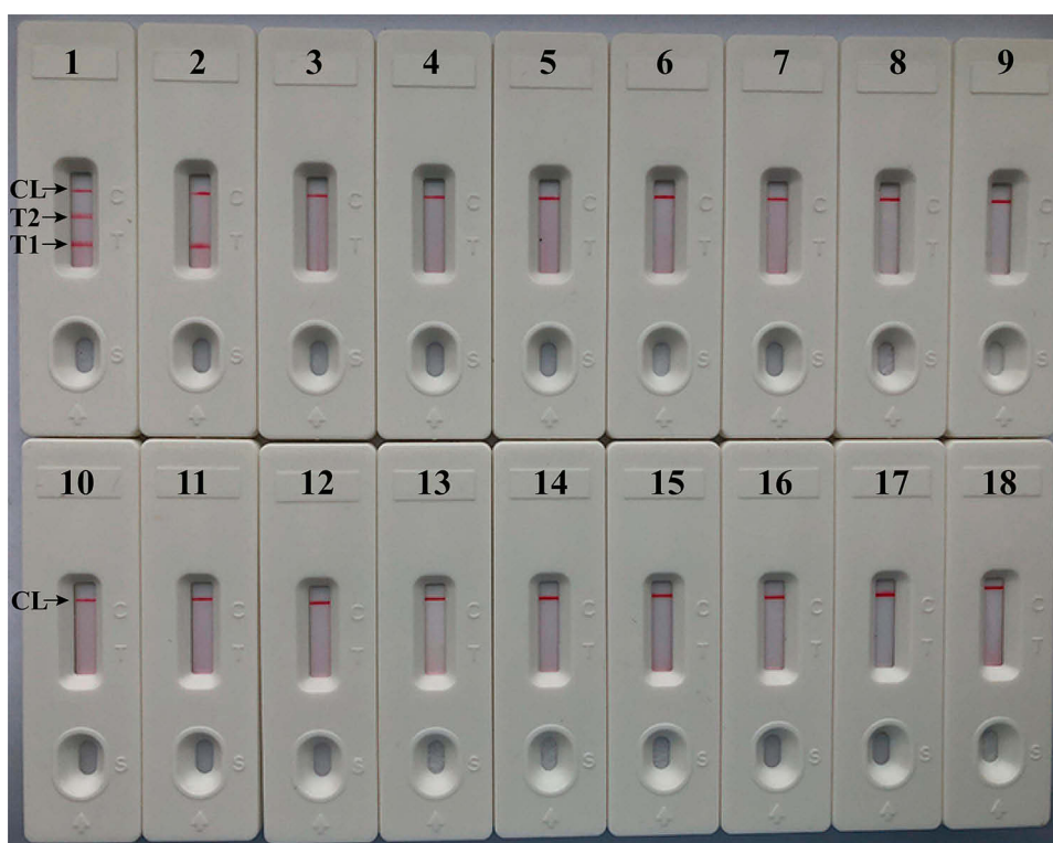
Figure 7 Analytical sensitivity of m-LAMP assay using different bacterial strains. The m-LAMP amplifications were performed using different genomic DNA templates and were monitored by means of visual format. Biosensor 1, MRSA (ATCC 43300); biosensor 2, MSSA (ATCC 25923); biosensor 3–17, biosensor 18, negative control (DW).
