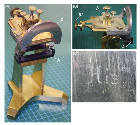
**Fig. 6.** The microtome of Wilhelm His. (A) Front view; (B) side view of stage; (C) engraved name 'His' on the strut. Background gridline spacing: 1 cm. The blade, held in the blade-holder h (fastened with wire for display purposes) is drawn downwards, the holder steadied against the flat face of g. Between cuts, the block clamped in h is advanced under the arch of h using the micrometer screw (h). Anatomisches Museum, Basel; photograph: M. K. Richardson.
