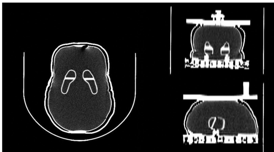
FIGURE 1 Overview of a striatal phantom. A striatal phantom consists of the left and right caudate/putamen and whole-brain compartments
