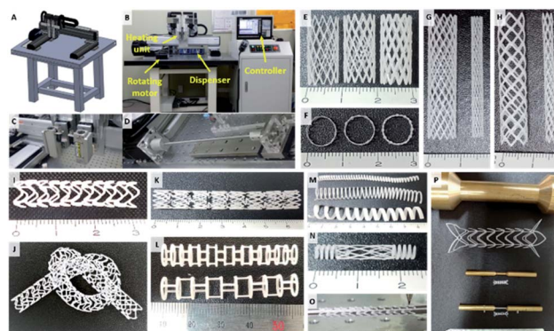
Fig. 2 (A) CAD image of Rotating rod combined 3D printing system (2RPS), (B) established whole system of 2RPS, (C) heating unit of 2RPS, (D) rotating unit of 2RPS, (E) various line width of stent (left: 300 \mu\text{m} /mid: 450 \mu\text{m} /right: 600 \mu\text{m} ), (F) various wall thickness of stent (left: 200 \mu\text{m} /mid: 300 \mu\text{m} /right: 500 \mu\text{m} ), (G) 12-peak stent with different stent diameter (left: 8 mm, right: 3 mm), (H) 6-peak stent with different stent diameter (left: 8 mm, right: 3 mm), (I and J) open cell type stent, (K) closed and open cell hybrid stent, (L) tubular type stent, (M) coil type stent, (N) coil, mesh hybrid stent, (O) protrusion surface imbedded stent for preventing migration, (P) various size of dumbbell type stent.
