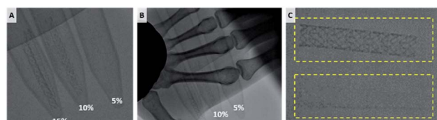
Fig. 5 Fluoroscopic image of contrast powder loaded BRS. (A) 5, 10, 15% iohexol loaded BRS. Visibility of the BRS (B) when covered with hand and (C) after washing (bottom).
