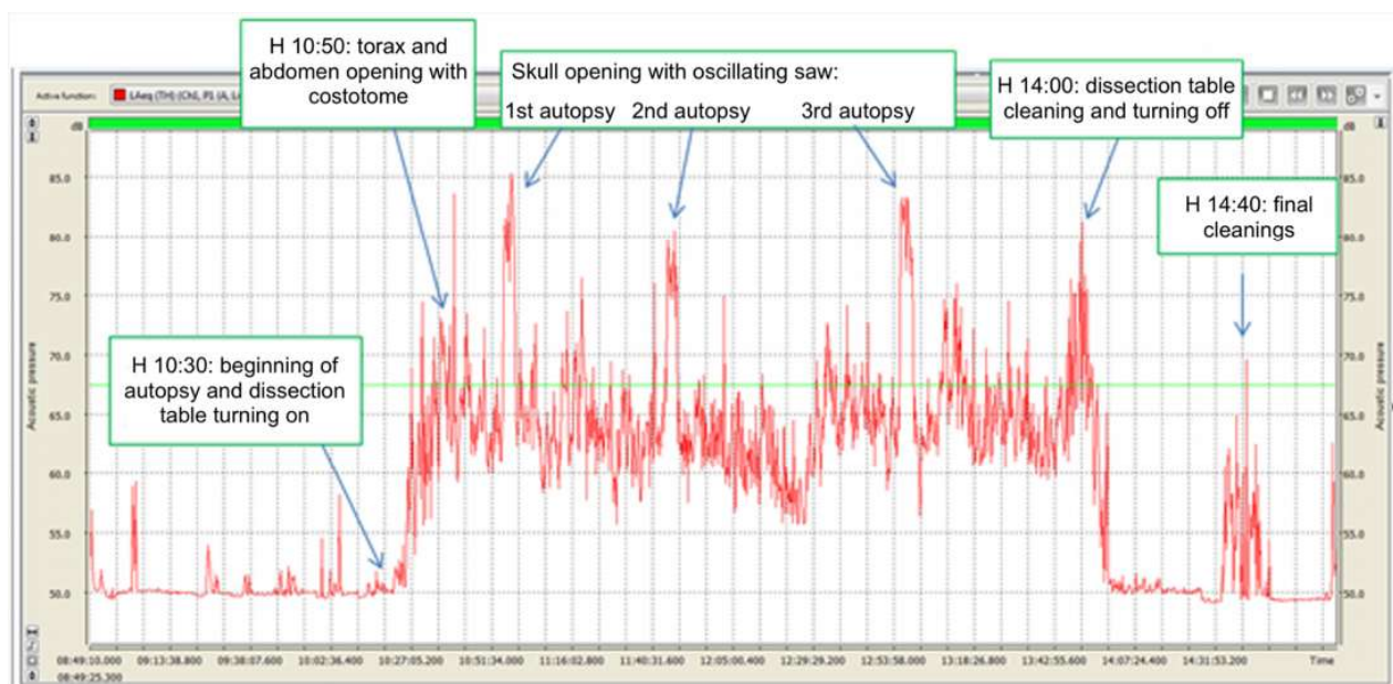
Figure 3. 30.09.2016. Acoustic emissions during 3 autopsies, each one performed on a different dissection table. Red line: equivalent sound level during T period of 15'' (Leg), expressed as dB (A). Green line: equivalent sound level during the entire monitoring period (Leg), expressed as dB (A).
