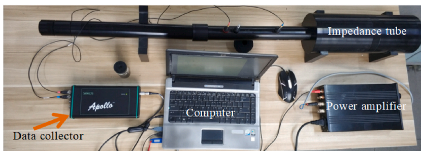
Fig. 4. Composition of sound absorption and noise reduction experimental test system.
