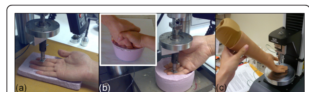
Figure 2 Setup for the indentation experiments (a) Flat-hand position, (b) Curled-fingers position, and (c) Prosthetic hand indentation. The Inset in (b) shows how the mould was prepared to restrict the hand in a typical handshake posture.
