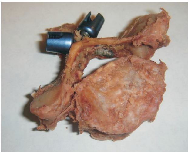
Fig. 2. Medial cortex breakage.
