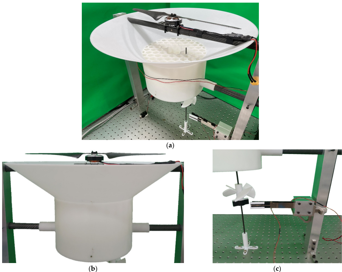
Figure 14. The assembly of the wind driven magneto-electric vibration energy harvester system. (a) brushless motor with a two-bladed rotor, (b) wind collecting cover, (c) windmill, and the magneto-electric VEH system.
