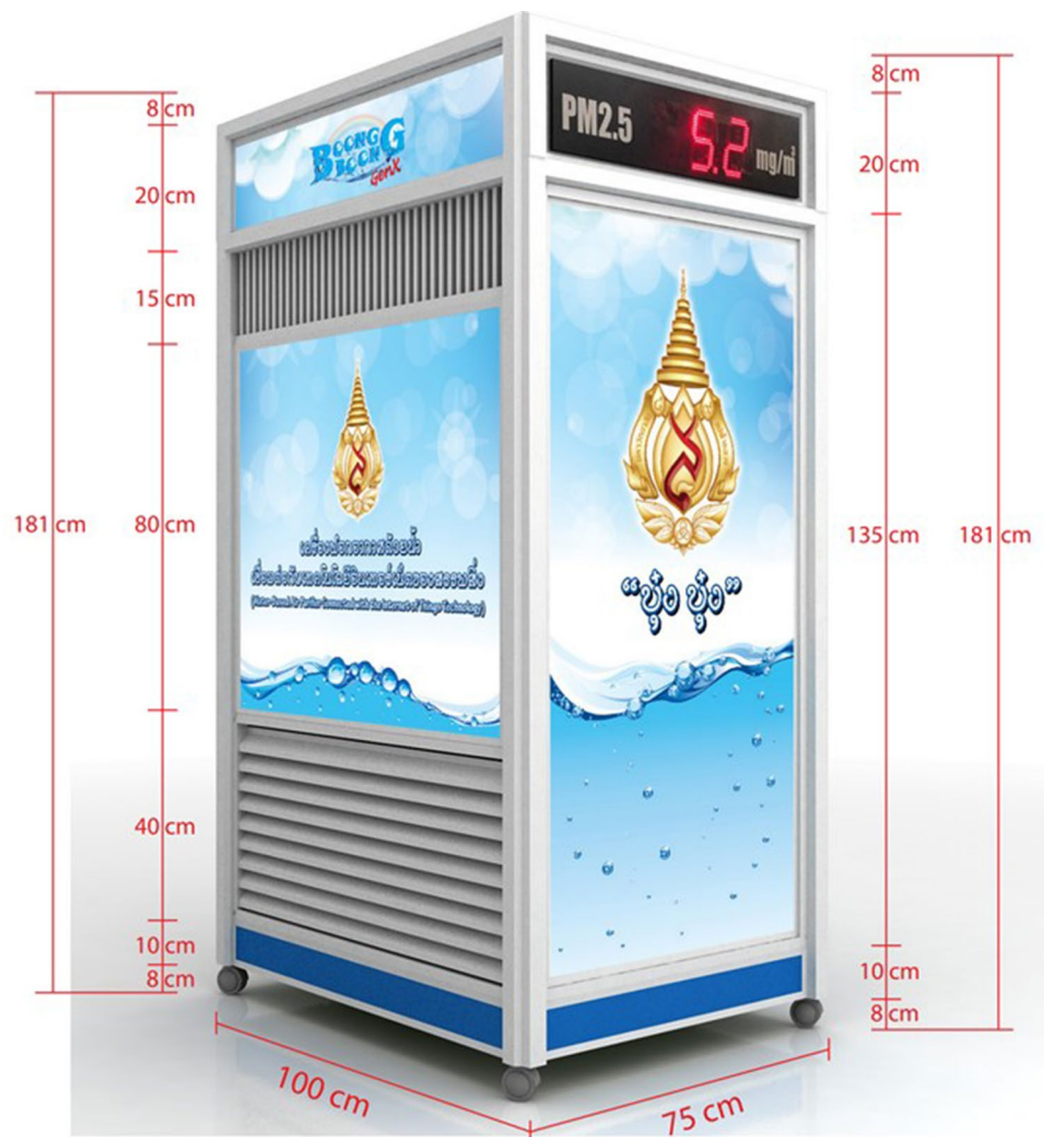
Fig. 1 Outer dimensions of water-based air purifier. Bottom grills serve as an air inlet, whereas top grills represent as an air outlet
