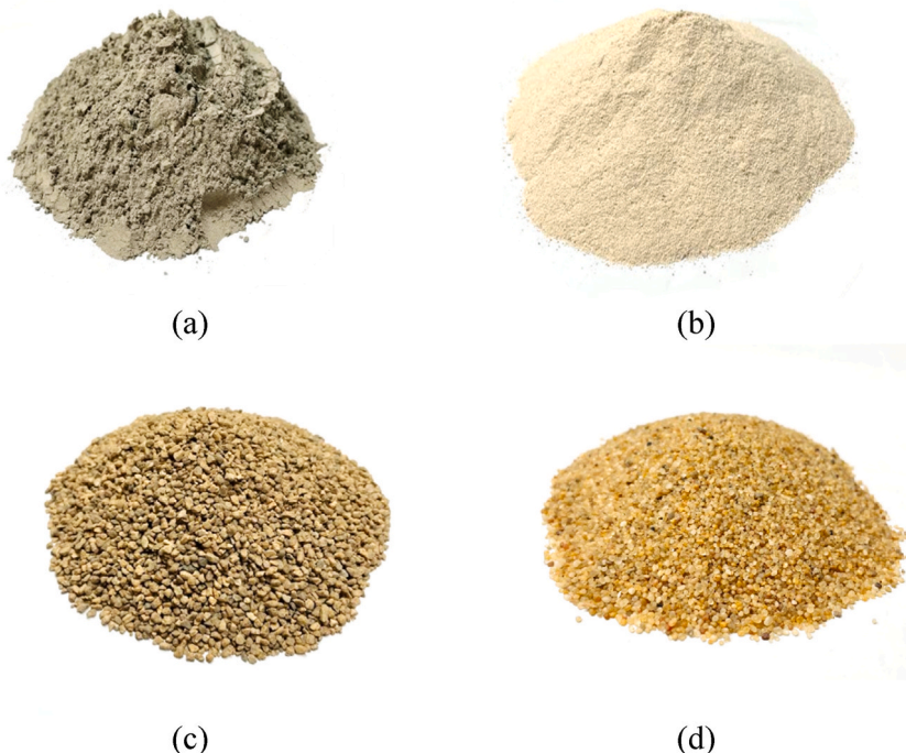
Fig. 1. Materials used for floor hardener as (a) Cement; (b) Fine sand; (c) Coarse sand; (d) Finer coarse sand.
