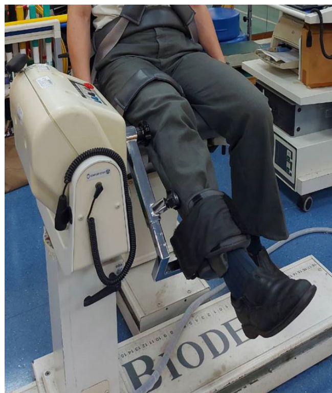
Figure 3. Exercise training (isokinetic or isotonic modes) using an isokinetic dynamometer.
