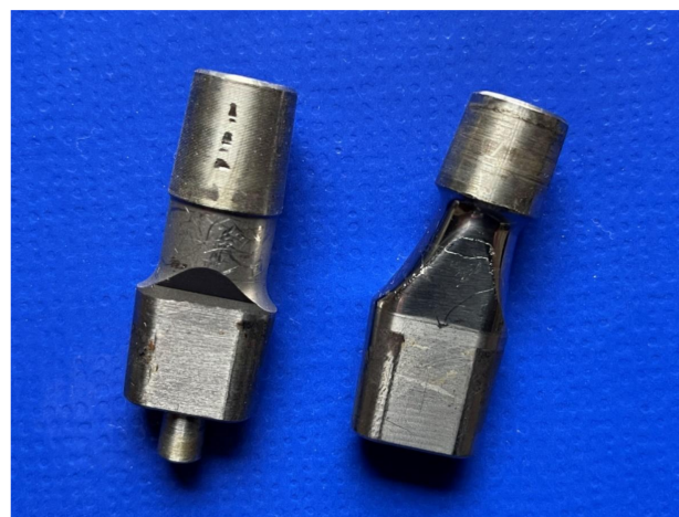
Figure 2. The interchangeable neck of the GSP (Cremascoli S.p.A.) ( left ) and Profemur Z (Wright Medical Technology Inc.) ( right ) dual modular hip implants. Both necks are short, the GSP-neck is straight, and the Profemur Z-neck is in an 8° varus orientation. The GSP neck was explanted 22 years after primary THA because of a late haematogenous infection, and the Profemur Z-neck was explanted 14 years after primary THA due to aseptic loosening. Note the same dimensions of the oval-shaped distal Morse taper.
