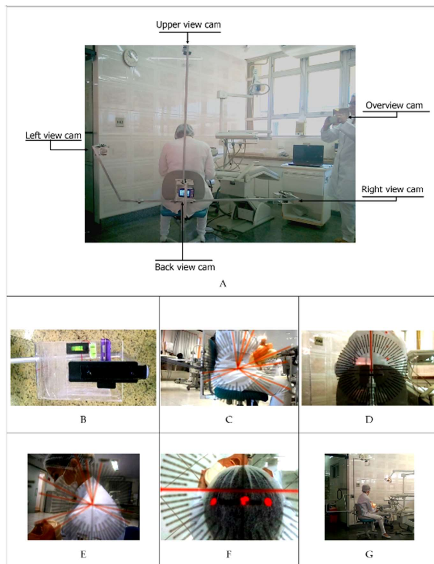
Figure 3. Device built to support cameras 1 to 4, camera 5 positioning and views obtained by each of the cameras. (A) Positioning of the 5 cameras; (B) Transparent acrylic support with the parameters and limits of angular inclinations and bubble levels to keep cameras straight; (C) Right view; (D) Back view; (E) Left view; (F) Upper view; (G) Overview camera.
